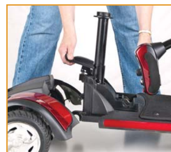
Step 3: Pull up on the drivetrain release lever to separate the front and rear frame sections!
